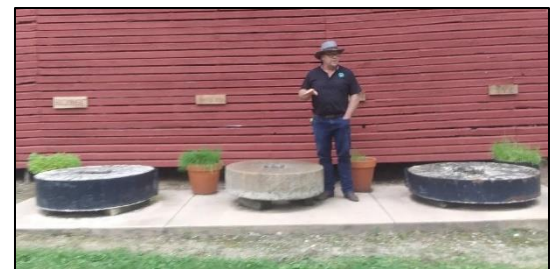
Two French buhr and one granite grindstone. In the background are samples of the different grains that are ground at Bonneyville.
